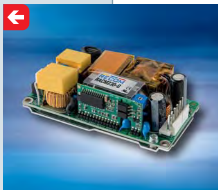
Contact cooled power supply with 230W peak power on 4"×2"
