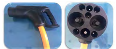
Fig. 7: Charging plug, where the temperature sensor could be installed along with the interconnection area to detect the abnormal temperature rise when charging.
